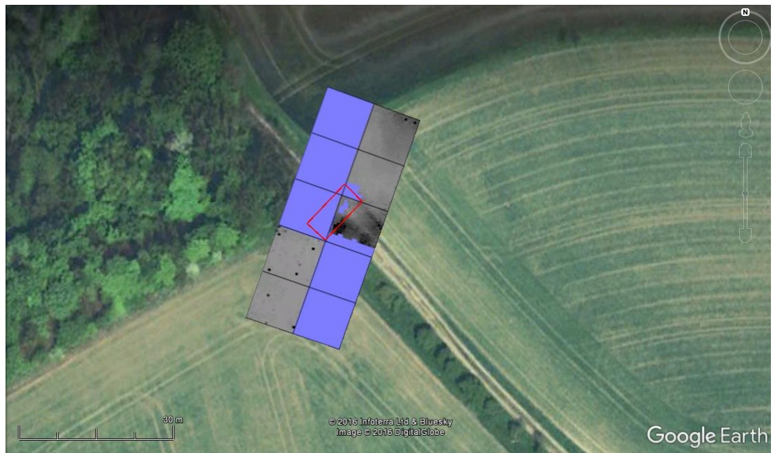
Figure 11 Electrical earth resistance survey of the area across Old London Road, indicating location of excavation trench (north to top)
